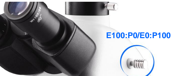
Trinocular Head Light Split Optional Between Switch E100:P0/E0:P100 & Fixed E80:P20 In Fixed Light Split, Eyepiece 80% : Photo 20% User Can View Image At Same Time In Both Path In Switch Light Split, Eyepiece 100%:Photo 0% / Eyepiece 0%:Photo 100%, Camera Can Have 100% Light For Photo Capture.
